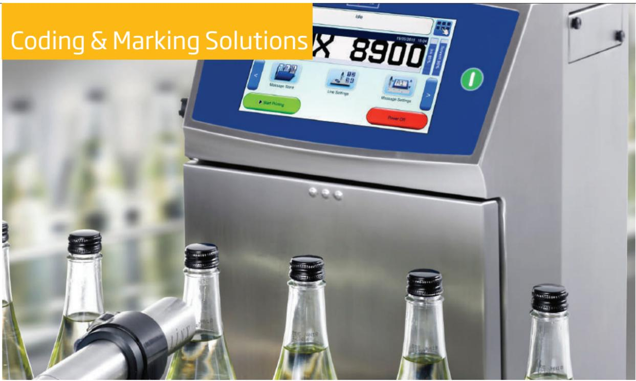
Linx Coders are used for coding and marking applications like sell-by-dates, manufacture dates, expiry dates, batching and other variable applications onto products.
