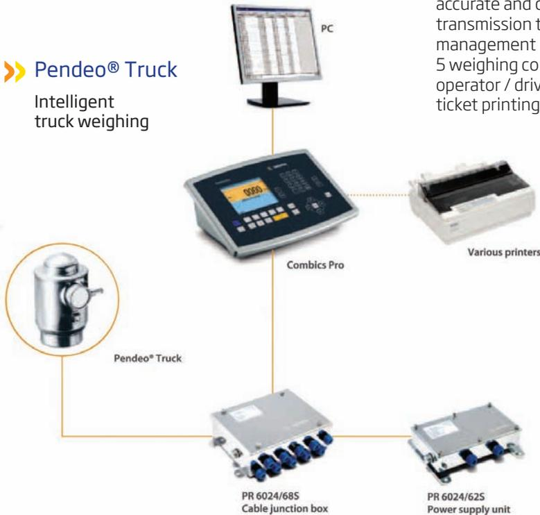
This system is 100% compatible with analog Minebea load cells with intuitive operation.
